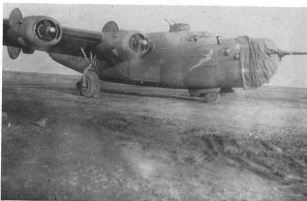
Broad Abroad undergoing pre-flight engine run up. Note the nose turret cover is still in place.
