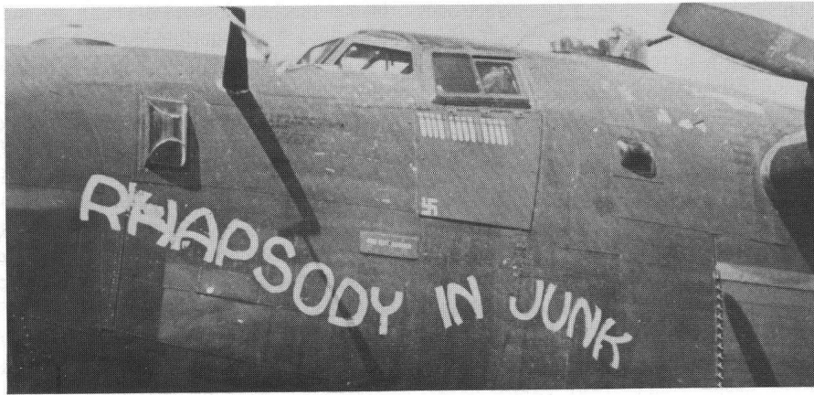
In an effort to reduce air crew losses, this B-24-H of the 309th Bomb Group, 8th Air Force received what appears to be a depot modification to the pilots center windshield panel and the sliding window by the addition of bullet proof glass. A slab of armour plate has been bolted on just below the pilots sliding window. Tony North photo.
