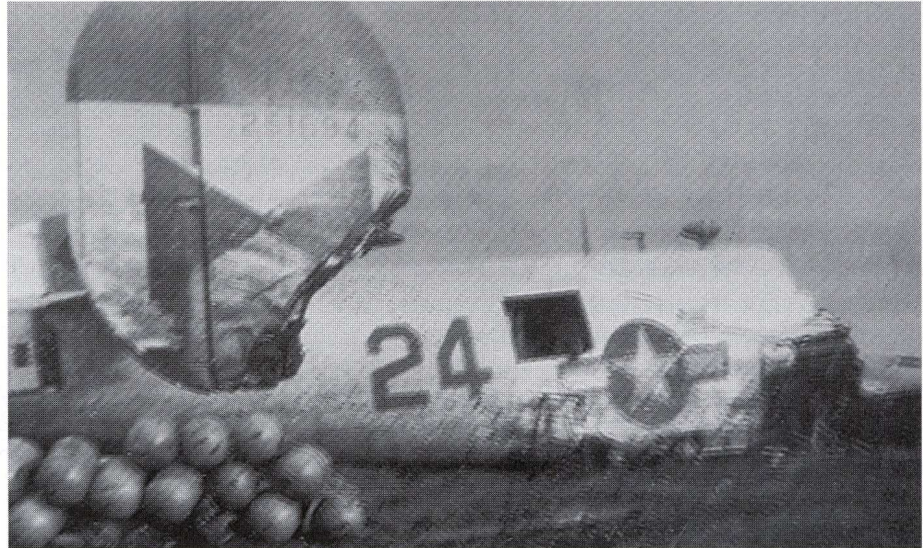
Plane 42-51694 nose no 24, showing battle damage to the right rudder after being dragged to the bone yard.
