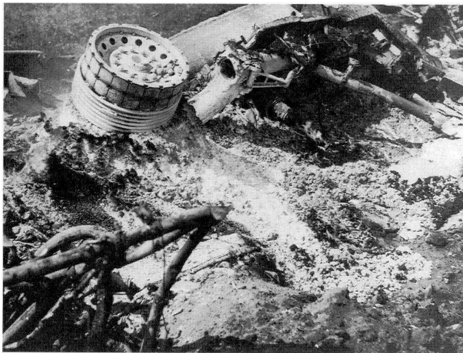
Part of a Main wheel showing the brake blocks
